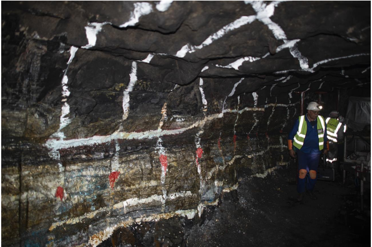
Figure 2: Gold reefs being marked up for trial mining
